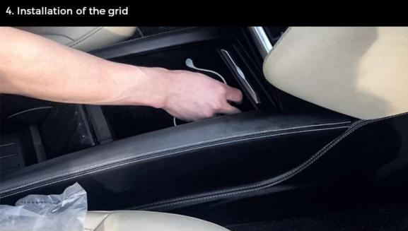
Note: When install it you may need to push it hard to insert the CCI (use a soft cloth to protect your armrest area), that is how CCI are designed otherwise it may shake or move when driving.
